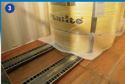
Lifting up goods directly from the floor
